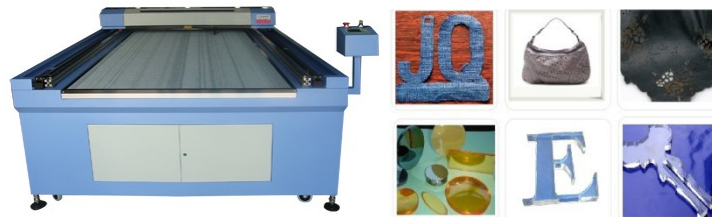
Figure 7 CO 2 Laser cutting machine with some output from non-metal materials
