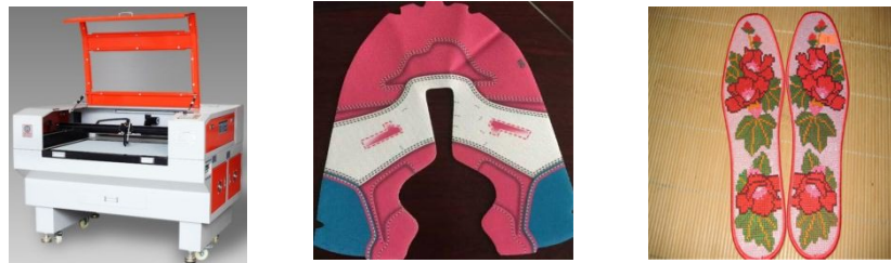
Figure 8 CO 2 Laser cutting machine and its output examples
